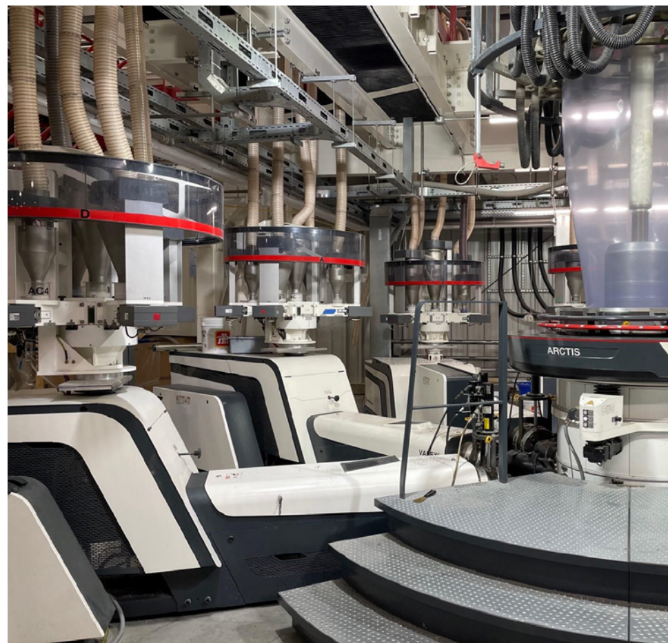
BMP Extrusion blowing 20% recycled content shrink film (above); 100% recycled content PET bottle with 20% recycled content film (right).
